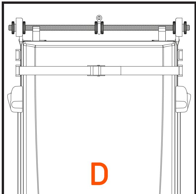
**DO NOT** hold winch head when raising or lowering the boiler.
