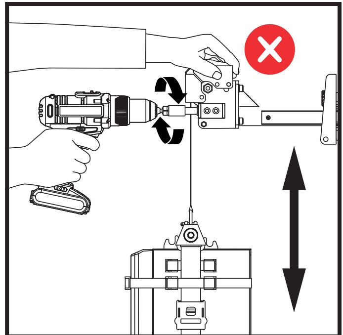
**DO NOT** winch a boiler unless the strap is vertical.
